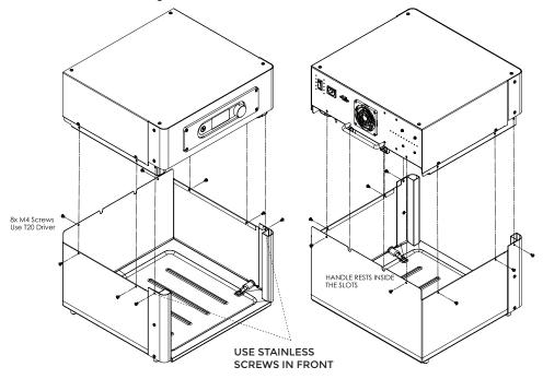
Pro Tip: Insert & lightly hand-tighten all screws before using T20 driver to fully tighten screws.
