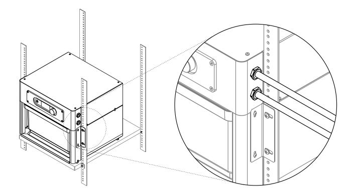
Depending on the size and desired spacing of your shelves or rails you may want to remove the rubber feet from the floor of the Z unit. Unit must sit level on the shelf without putting pressure on front lip and without support from the stabilizing brackets.
