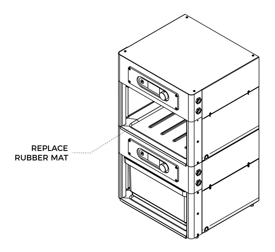
**05.** Stack the Heating Module on top and finish assembly just as you did with the first unit.
