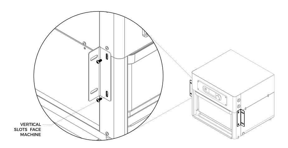
Pro Tip: Don't fully tighten these screws until unit is mounted in its final position on rack.
