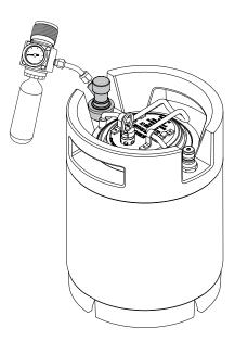
Attach the Party Tap to the Brewing Keg by connecting the black ball lock connector to the Brewing Keg OUT post.
