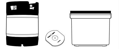
Check that the Water Reservoir stopper is in place. This is located in the Water Reservoir in the center back area. Add 0.5 gallon (or 8 cups) of distilled water to the Water Reservoir. Add about 0.5 gallon of clean tap water to the Brewing Keg. Place black Keg Seal over the opening of Brewing Keg and press into the center of it until it pops into place.
