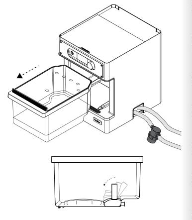
Place food bag(s) in Step Filter. If using a Ziploc<sup>®</sup> bag, place bag(s) against the side of the Step Filter with the top hanging out over the edge of Step Filter. Once you place the Step Filter lid on it will clamp the bag(s) into place. Vacuum sealed bags should sink to bottom. If necessary, place a foodsafe object on top of bag(s) to make sure they will stay fully submerged in the water during the entire
