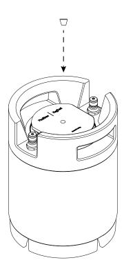
Set the Brewing Keg aside to cool overnight in room temperature and remove the Keg Cozy from the Brewing Keg. It is normal for the Keg Seal to suction slightly into the Brewing Keg as it cools, don't worry it will not be pulled all the way inside. You will need to pitch the yeast within 24 hours after brew session is completed.
