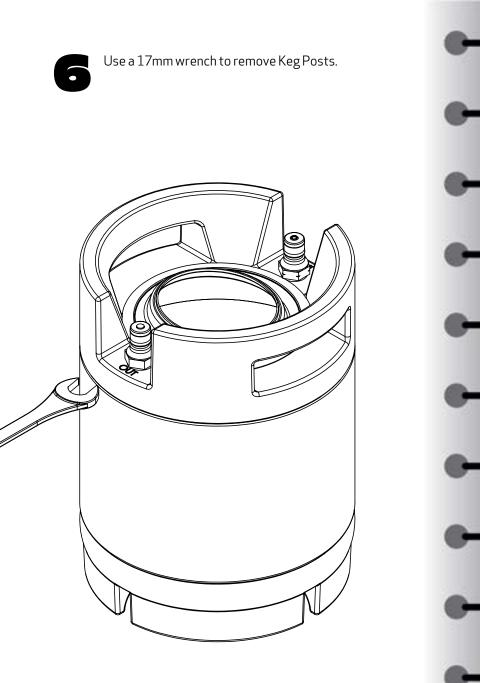
**CAREFUL!** There is a metal spring and valve inside both the IN and OUT post Ball Locks, this is called the Poppet Valve. It may jump out as soon as the IN or OUT posts are taken off. Make sure you are standing over a contained area, not a sink with an open disposal or drain, nor a patterned carpet.
