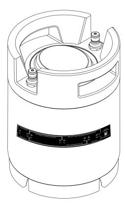
Remove the black Keg Seal and Stopper from the Brewing Keg.
