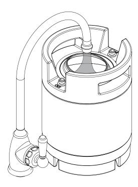
Place the black Keg Seal on the top of the Brew Keg opening, push in the center until it pops into place. Make sure the hole in the center of the Keg Seal is open. Pull the Keg Cozy over the Brewing Keg. Attach the BLACK Ball Lock Connector hose connector to the Brewing Keg post marked "OUT". Repeat the procedure with the GRAY Ball Lock Connector hose (capitalize) on the brew keg post marked "IN".
