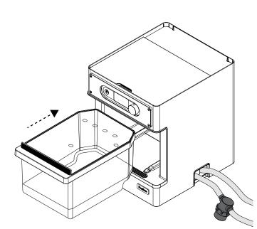
Make sure your keg is properly connected and filled with 5 quarts of water, press the Control Knob to continue to the next step.
