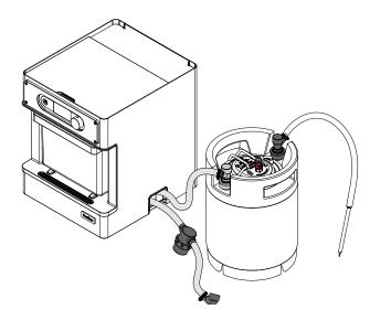
Direct the Bottling Tube to the bottom of the sanitized bucket and press down. Press the Control Knob. The initial beer coming from the Bottling Tube may contain trub (sediment). When no more trub flows in to the waste container press the Control Knob to stop the drain, this should take no more than 30 seconds.
