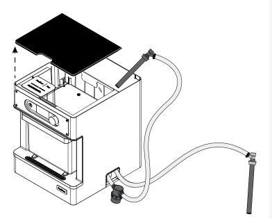
Unscrew and remove the Inline Filter cap. Remove the blue filter insert and rinse it thoroughly using tap water. Place it back in the Inline Filter and screw the filter cap back on, finger tight.
