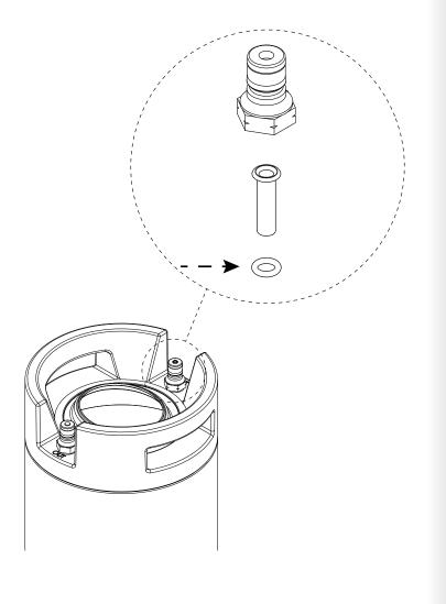
The OUT post is connected to a long Dip Tube that reaches the bottom of the keg. Remove the black O-ring attached to this tube.
