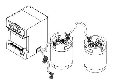
Press the Control Knob to begin transferring beer from the Brewing Keg to the other Brewing Keg you will use for serving. When racking is complete, the Transfer Tube will blow empty. Press the Control Knob to turn off the pump and stop the process. Disconnect the GRAY ball lock connector from the Brewing Keg IN post and the BLACK ball lock connectors from the OUT posts of each keg. Turn the Gray Pressure Relief Valve back 90 degrees to close.
