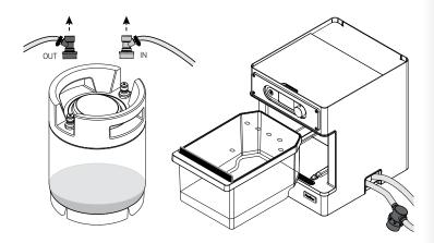
Connect a clean Keg Wand to the BLACK Ball Lock Connector by pulling up on the outer ring of the Connector and inserting Keg Wand, release outer ring and make sure it is securely connected to Connector. Press Control Knob to begin pumping water out of Water Reservoir and into the Step Filter. Follow on-screen instructions and press Control Knob between steps. Press Control Knob when the Water Reservoir is empty.
