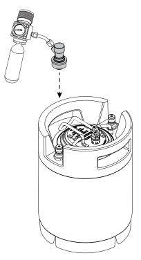
Place the Brewing Keg with attached CO<sub>2</sub> Regulator into your refrigerator to chill and carbonate for approximately 36 hours.
