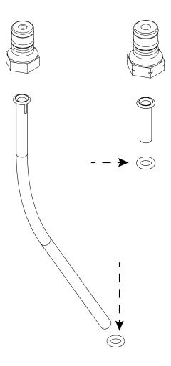
Make sure the IN/OUT keg posts are on the correct sides and are tightened down. Remember, the tube for the IN post is shorter than the Dip Tube for the OUT post. The Dip Tube is slightly angled and the end of it should almost touch the center of the bottom inside the Brewing Keg.
