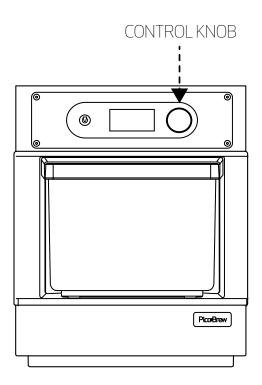
Remove the Water Reservoir lid. Insert the end of the BLACK Ball Lock Connector ("OUT") Keg Wand into the Water Reservoir. Run the pump until the Reservoir is drained. When the Reservoir is empty stop the pump by pressing the Control Knob.
